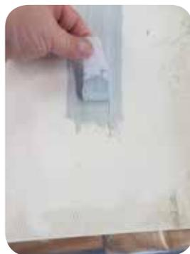
Silicone-based Roof Patch adhesion to aged TPO
