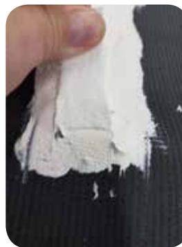
Repair Hero adhesion to aged reinforced EPDM
